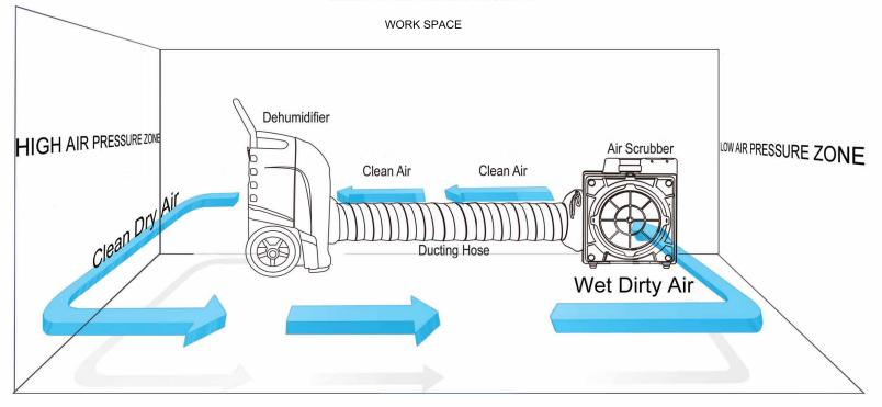
XPOWER's XD-125 is part of a revolutionary new Air Purification & Drying System which uses the combined power of the Air Scrubber and Dehumidifier to remove moisture and contaminants from the air!
